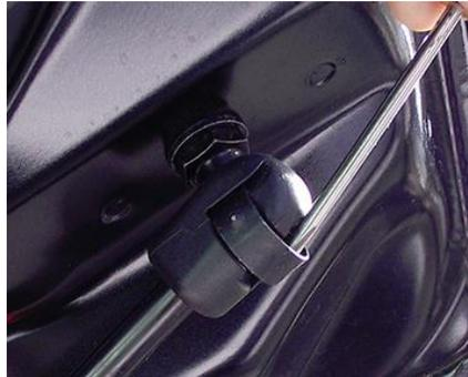
4. Rotate the gas strut toward the front of the vehicle and rest it on the radiator core support inboard of the hood rests. This will keep it out of the way as you work on the hood. You can close the hood momentarily.
