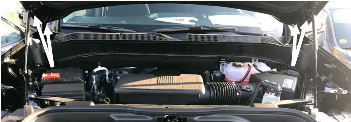
2. Place masking tape along the hood hinges (shown below) to ensure proper alignment.
