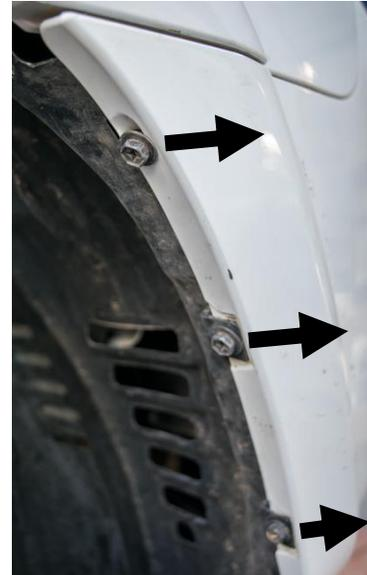
7. This will be the last step before the entire front clip will come off. Prepare a safe area to place the removed front clip. Remove the left and right plastic fasteners using a Standard screwdriver, shown at the top and bottom of the picture to the right. Prepare to support the front clip while removing the center bolt with the 10mm socket wrench. Once removed, place front clip away from the vehicle.
