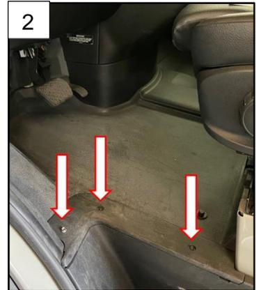
3. Using a T30 torx, loosen the 4 bolts holding down the battery cover and slide the battery cover to remove.
