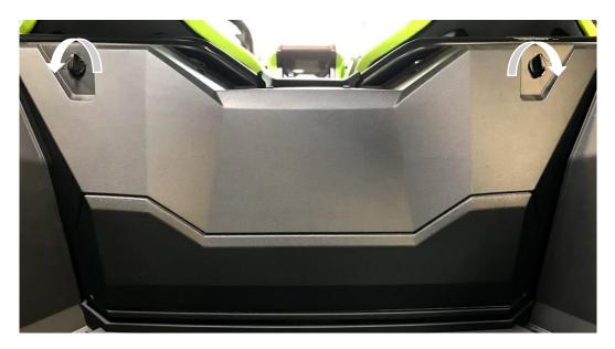
5. Unpin the grey clip on the left edge of the back panel circled below. Disconnect the plug. With the Honda Talon RTL adapter (sold separately from RTL harness), plug it into each respective plug. The grey clip can be moved to the new adapter plug if desired. Place clip back into the original location.
