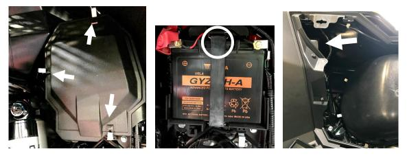
7. Remove the in-cabin rear access panel by pulling the top edge toward the front of the vehicle (see image on left below). The picture on the right below shows where the reverse light switch leads can be routed (Turn signal switch also if purchased). The switch can be removed to route wires through and then reattached. Take note of switch terminal configurations.
