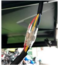
12. There are two wires with female bullets along the harness nearest the four female bullet connectors. Connect those wires (yellow, red) to the corresponding colors on the inline adapter from step 5. Close the rear cargo cover.
