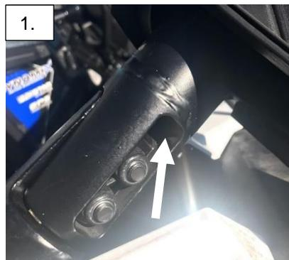
2. The exit is on the passenger side cage tube adjacent to the front crossmember.
