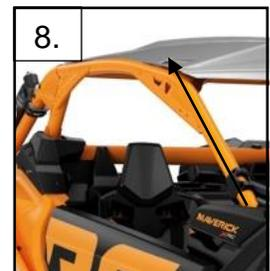
Re-torque all the fasteners after 100 miles.
