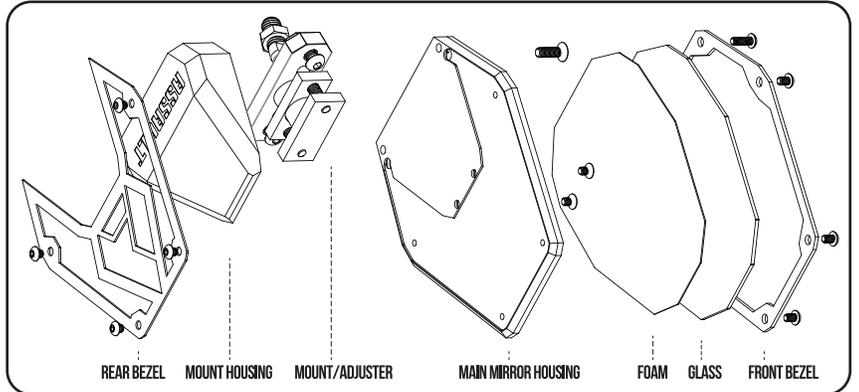
REAR BEZEL MOUNT HOUSING MOUNT/ADJUSTER MAIN MIRROR HOUSING FOAM GLASS FRONT BEZEL
