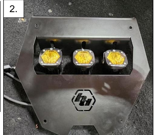
3. Locate the included 2-pin splitter and plug it into the 2 outermost S1s.
