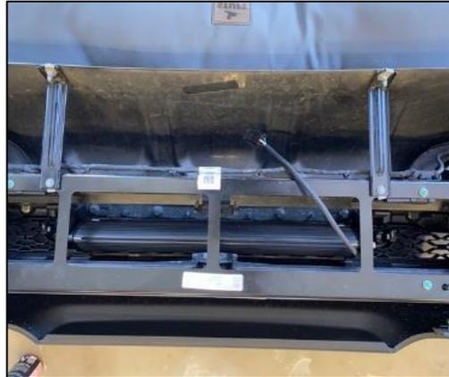
10. Using the existing hole location, Mount the bracket with the supplied 1/4-20 hardware.
