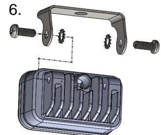
7. Mount the new fog lamp assemblies into the fog mounting bracket with two of the four screws from step 5. Repeat for the other side.
