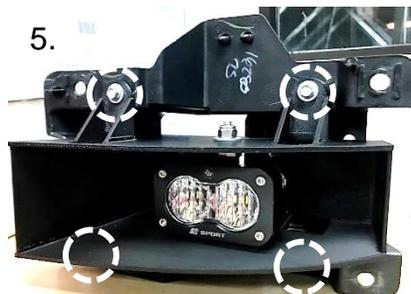
6. Assemble the S2 lights to their brackets with the provided hardware and 4mm Allen wrench. Remove bezel bolts with the 2.5mm Allen wrench and rotate the bezel 180 degrees. Tighten bezel bolts. With the 1/4" hardware and 7/16" wrench and socket, mount the S2s into the Baja designs fog light bracket.
