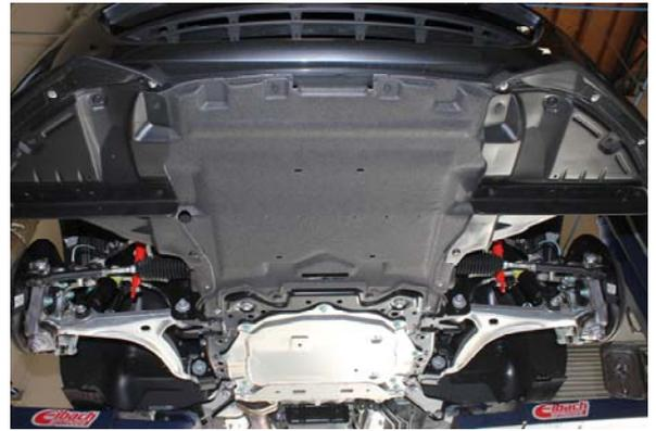
12. Double check to make sure everything is properly positioned and tightened, then, reinstall the inner fender valances and the underbody splash shields.
