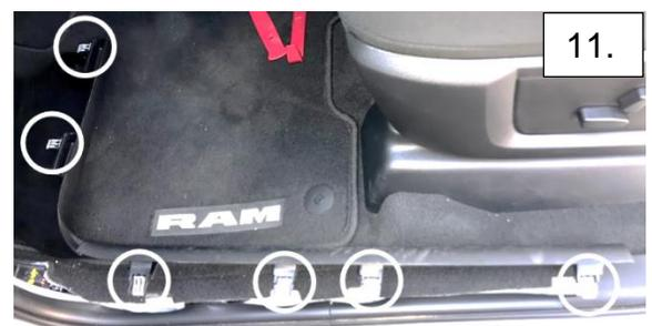
11. Unclip the flap next to the parking brake pedal. Carefully pry the six lower door sill trim clips. (Trim is shown removed for detail)
