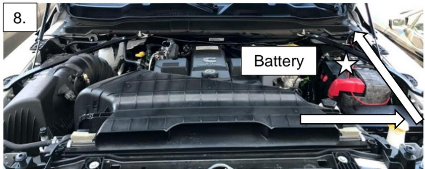
8. Following the path shown, attach the battery leads of the harness to the battery (starred) and mount the relay to a nearby bolt.
