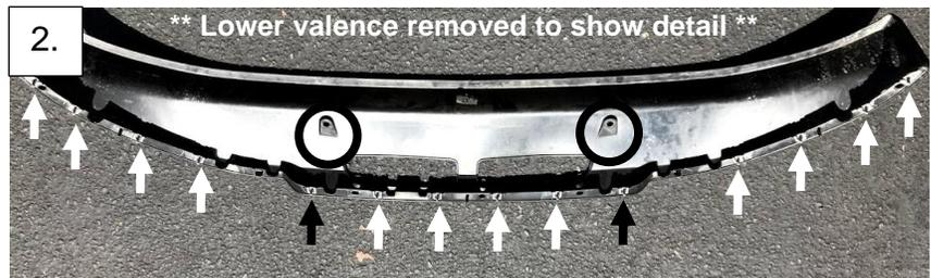
3. Remove nuts on the backside of the bumper in the black starred locations with an 8mm wrench. Place the 1/4" bolts with washers in the empty holes on the backside of the bumper in the white starred locations. The bolt heads should be facing the front of the vehicle.
