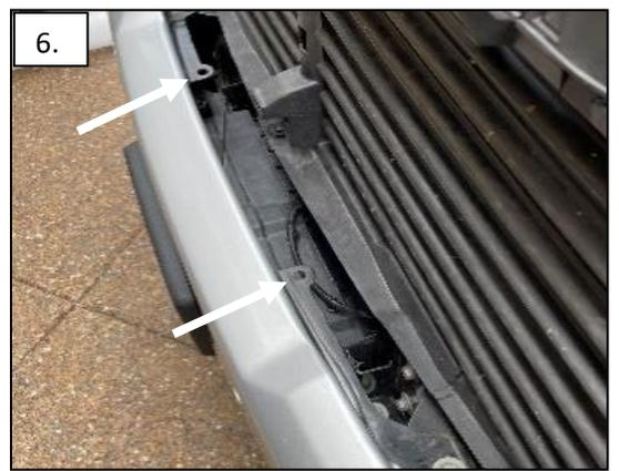
7. Mount the 2x brackets with the supplied hardware onto the bumper. Use EPDM rubber on brackets if needed. Place the light bar between the brackets. Slide the brackets to the mounting tabs on the light bar. Using a 7/16" wrench, lightly tighten the light. Center the light to the vehicle, finalize torquing down the brackets.
