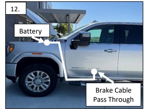
13. On the bottom of the floor is the brake cable pass through, Route the switch lead through it to the inside of the cab.
