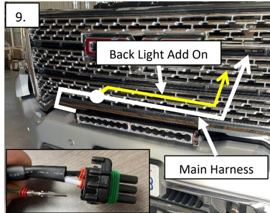
10. Route the main harness and back light add-on harness to the battery. Using a 10mm socket, mount the 3/8" Red wire ring terminal to the battery. Using a 13mm socket, mount the 3/8" black ring terminal to the battery cradle.
