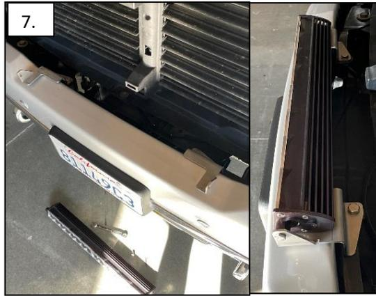
8. Remove the light from step 7. Re-mount the grille.
