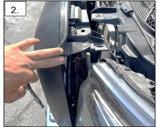
3. With step 2, push on the top of the 4 self-locking tabs allowing the grille to be removed.
