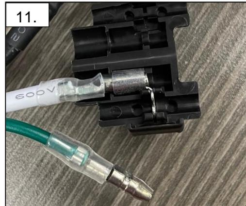
12. Place the brown up-fitter wire into the splice connector attached to the white wire and close the plastic housing. Connect the fuse tap to the green wire with the female side of the bullet connector. Apply heat to the clear heat shrink to protect the bullet connectors.
