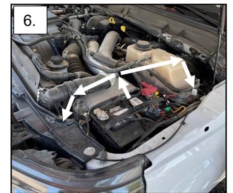
7. Route the wires as shown behind the headlight & bumper. Keep away from any sharp edges.
