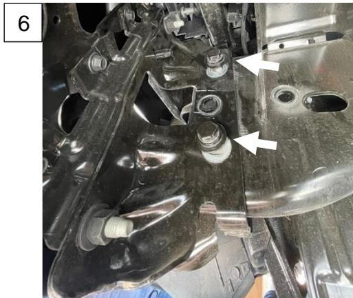
7. With an assistant, support the bumper on both sides and remove the remaining bumper mounting bolts. Place the bumper down onto a soft work surface.
