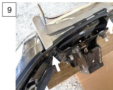
10. With a razor knife, trim the weather seal along the dotted line as shown to allow space for the bracket. Install the weather seal fasteners. Push the bracket down against the bumper and tighten the bolts with the 13mm socket. Repeat steps 9-10 for the opposite side. Reinstall the bumper back onto the vehicle by following steps 2-7 in reverse.
