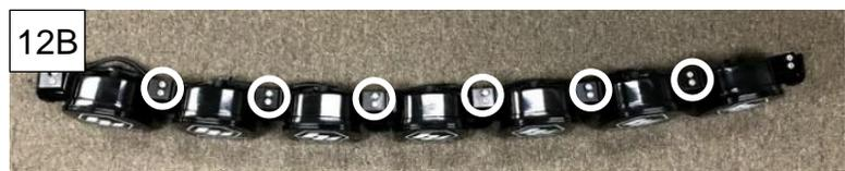
13. Mount the light to the brackets using the provided Allen wrench, 7/16" socket wrench, and the provided hardware. Loosen the center light housing bolts enough to slide the support brackets. Have an assistant pull up (0.25"-0.5") on the light and slide the support brackets down and back until they contact the bumper. Tighten the housing bolts.
