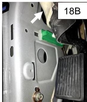
20. Drill 3/4" hole in desired dash location. Mount switch and reattach wires. Tie all wires away from any hot and/or rotating components.
