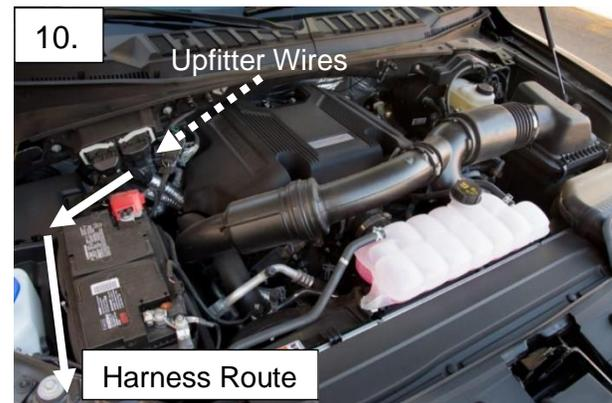
11. Locate the bundle of upfitter wires on the passenger firewall taped to the harness passthrough closest to the motor (Dotted arrow). Do not use the bundle of wires that is furthest from the engine (Left arrow).
