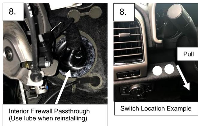
Tie all wires away from sharp, hot, and/or rotating components.
