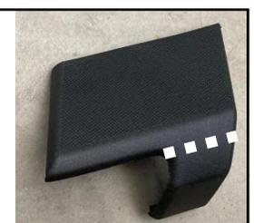
10. Open the hood. Unravel the harness and route the light lead of the harness down behind the passenger side headlight (also behind the air cleaner). Pull the white arrowed top edge of the seal out from the fender across to the grill.
