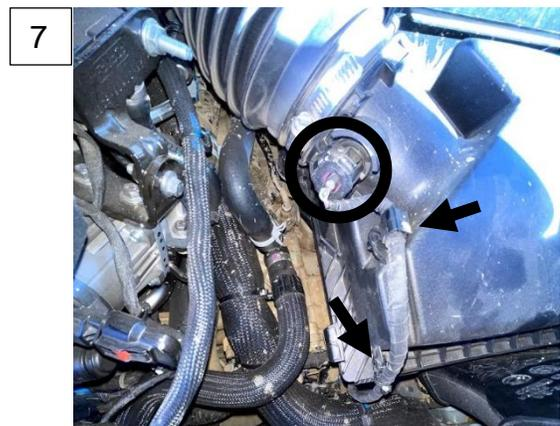
8. Loosen the circled battery clamp fasteners with the 10mm socket with the extension. Remove the battery terminals (+/-) with the 10mm socket and place them aside; black lead first. Now the battery can be slid forward and removed for the moment. Remove the arrowed firewall grommet and route the harness switch lead through. Pull enough slack in from inside the cab to reach the headlight controls.
