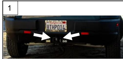
2. Assemble the two L-brackets onto either side of the receiver hitch using the provided hardware.
