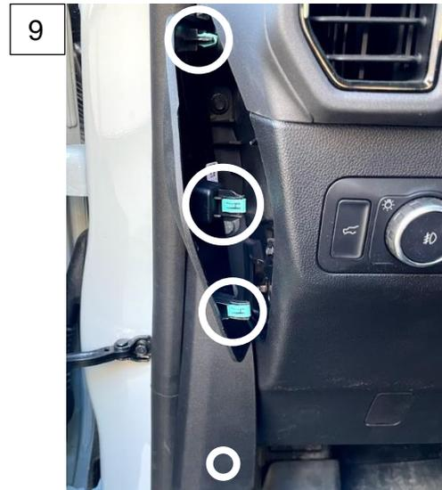
10. Carefully pull the edges of the headlight control dash panel until the clips release. Remove the arrowed headlight control unit connector.
