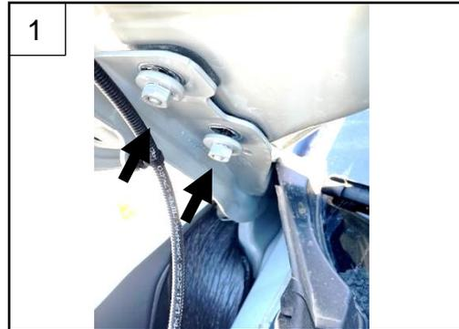
2. Place the passenger side bracket over the bolts and tighten the nuts. Repeat for the driver side.
