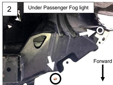
3. Reference the image on the right looking up from under the front bumper on the passenger side. Pull the inner fender towards the rear of the truck to expose the area behind the fog lights. Locate the outer passenger side bumper mounting bolts and remove with the 14mm Socket wrench.
