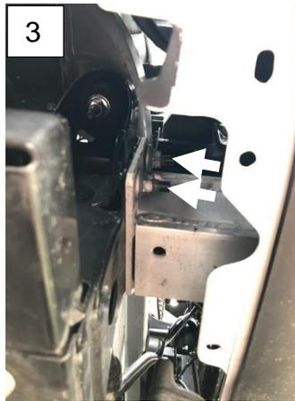
4. Locate the passenger side Baja Designs Tacoma Linkable bracket. Reference the image on the right. Find the slotted preload base bracket.
