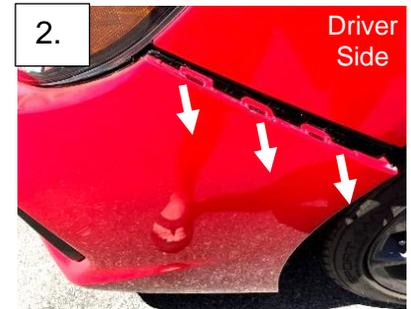
2. Along the bottom front edge of the front clip, there are seven more plastic fasteners that will need to be removed with the Flathead screwdriver in the same manner. Then, pull each side of the front clip gently until the panel releases as shown.
