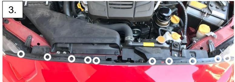
4. Assistance recommended for this step. Remove the last fastener in the top edge of the hood seal and remove the hood seal strip. With assistance, carefully pull the front end away from the vehicle enough to reach the fog light connectors. Unplug the fog lights (if present). Unplug the front camera (if present). Now, place the front clip aside on a soft surface.
