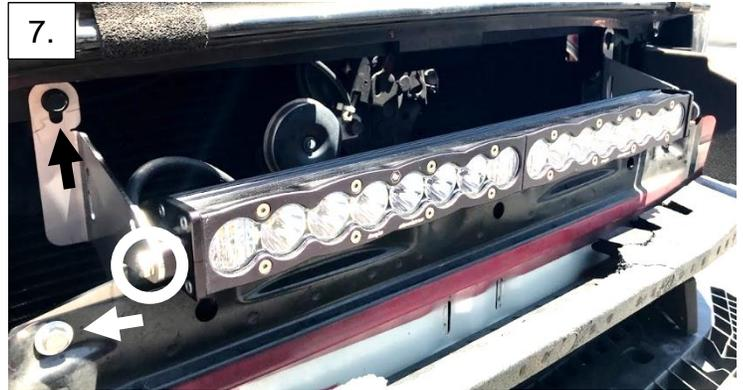
8. Place the front clip back onto the vehicle to check the placement of the light. The light can be adjusted vertically if desired. Repeat as necessary. Once satisfied, remove the clip, and tighten all the hardware. Route the power cord up through the radiator cover opening on the passenger side.
