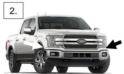
2. Assistance recommended for this step. Gently pull the trim under the grill starting in one wheel well, then the opposite side. Place the entire piece aside on a soft surface.
