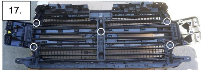
17. Place the grill/shutter assembly face down on a soft work surface. Tighten the four 10mm nuts and center 10mm bolt from step 9. Replace the splash guard from step 8.
