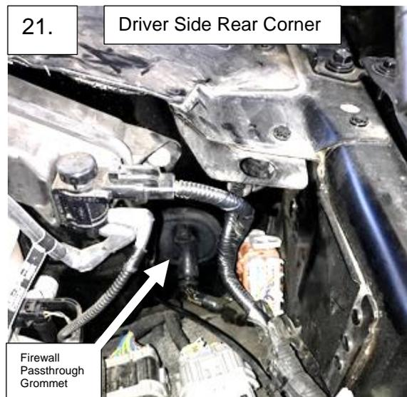
21. Locate the firewall passthrough grommet and gently pull it away from the firewall. Cut the zip tie on either side holding the wires together.
