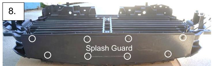
9. Remove the four circled 10mm nuts on the gold studs shown. Note: if the nuts just spin, move on and this will be addressed in step 11. Remove the center circled 10mm flange head bolt. The XL trim level grill will differ slightly.
