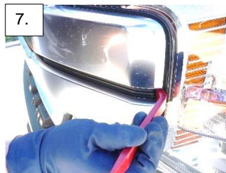
7. Assistance recommended for this step. Pry each side of the grill with the trim tool to pop out the sections next to each headlight. Pull forward to remove the grill and place it on a soft work surface face down.
