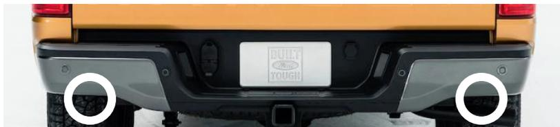
2. Below on the left is an image of the driver's side mounting location behind the bumper. Using a 13mm socket wrench, remove the bolt, place bracket onto the mount as shown below on the right, and lightly tighten. The single hole on the brackets should be oriented toward the sides of the vehicle. Repeat for passenger side.
