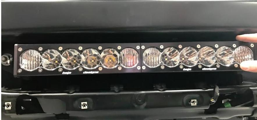
7. Once satisfied with the positioning of the light, tighten the 1/4" hardware, then tighten the large factory nuts from step 5.
