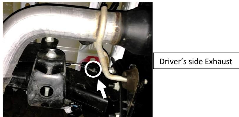
9. Plug in the weatherpak connector on the upfitter harness to the splitter going to the lights.
