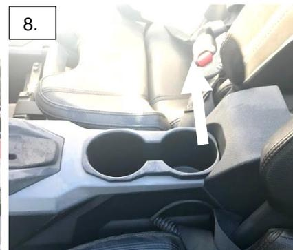
8. Pull up on the back of the cupholder and remove.
