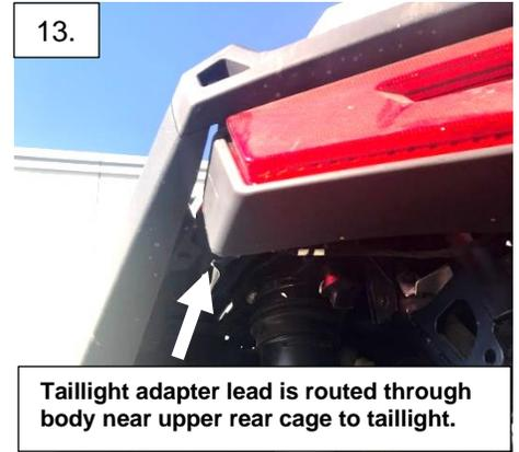
14. Disconnect the driver side taillight connector and plug in the Baja Designs in-line taillight harness adapter to the plug and the taillight.
