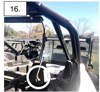
16. Crimp the RTL power cord wires with the provided male bullet terminals and covers. Attach the RTL harness to the RTL. Tie all wires away from sharp, hot, and/or rotating components.
