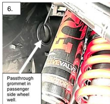
6. Route the light plug lead of the wiring harness from the passthrough in the passenger wheel well to the opening under the hood along the white arrow in the second picture.
