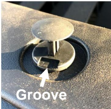
Using the Flathead screwdriver, remove the two plastic fasteners circled above. To release, pry up the head in the groove pictured on the left. Then pry the entire fastener out and set aside.
