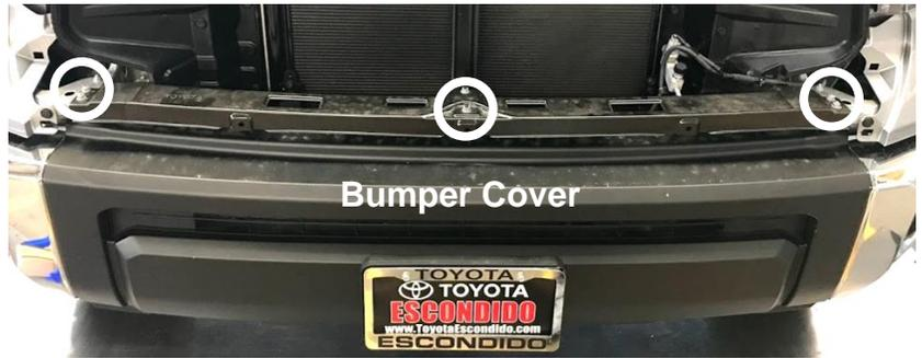
5. With the 10mm socket wrench, remove six bolts arrowed below. Leave the plastic fastener in the center until step 10.
