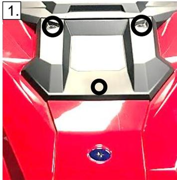
2. Unclip the front cover/camera and carefully rotate counterclockwise and let it hang over the grill. **Do not pull on the wires!** Remove circled bolts with the T40 Torx bit. Unclip the arrowed plastic fastener with the flathead screwdriver. Remove the Passenger side T40 and plastic fastener.
