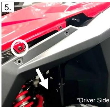
5. Carefully pull the fender down to expose the circled T40 Torx bolt. Remove.
