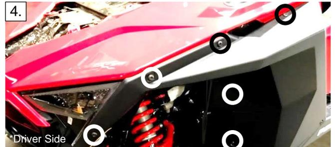
4. Remove the T40 Torx bolts on fender in the circled locations shown.
