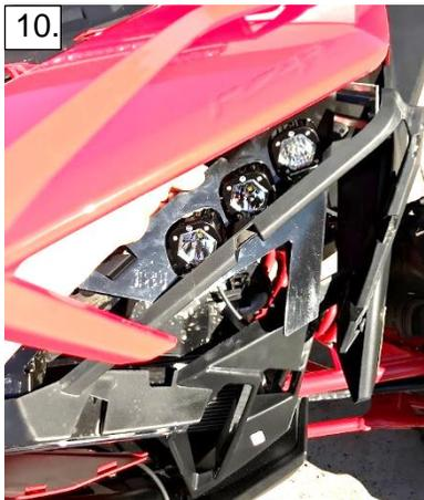
11. With the OEM T25 Torx bolts and the provided washers and bushings, attach the headlight assembly to the headlight frame. (Note: Bushings go behind the bracket, not inbetween bracket and mount).
