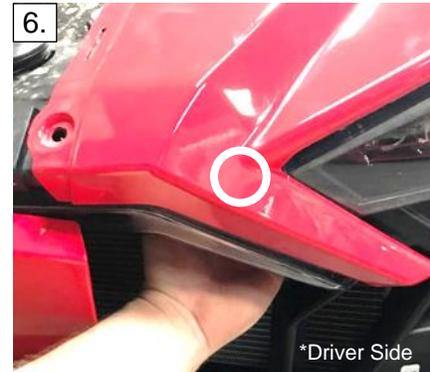
6. With the T25 Torx bit, reach through the grille to remove the inner headlight mounting bolt. **Use care not to damage radiator fins.**
