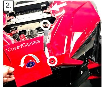
3. Release and remove the grille by pulling the two circled tabs downward.
