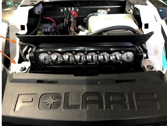
6. Using a 10mm socket and connect the negative and positive terminals of the wiring harness to the positive and negative terminals under the hood or directly to the battery underneath your seat. Do not connect the harness leads to the far left terminal (this can only take a small amount of amps)
