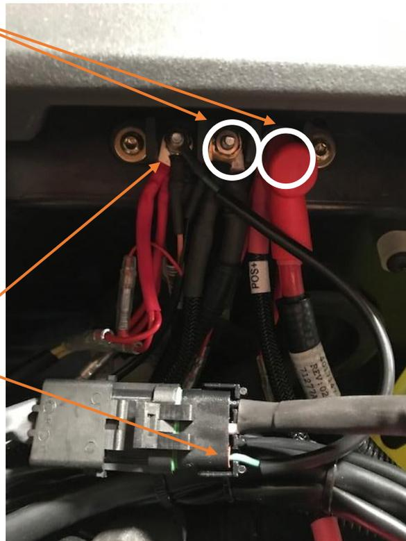
7. Insert the S8 backlight extension into the empty slot on the harness and attach that to the FAR LEFT terminal post to enable the back light feature to come on with ignition.
