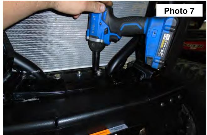
5. Install the hawse fairlead using the hardware supplied with the winch. **See Photo 7.**
