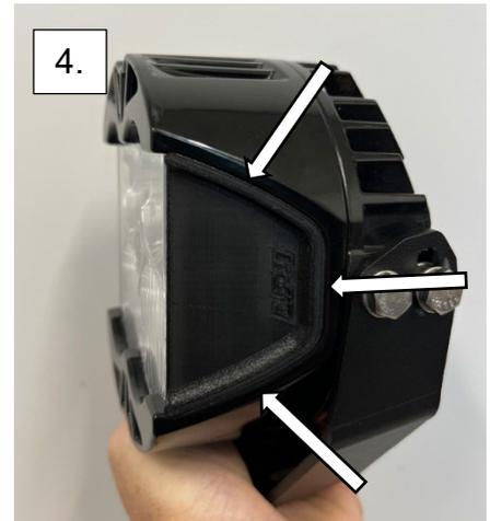
4. Before applying the IPT cover to the outside of the lens. Push the IPT cover to the edges of the light housing then apply pressure to the IPT cover to secure the cover to the lens. (this light will be mounted on your passenger side)
