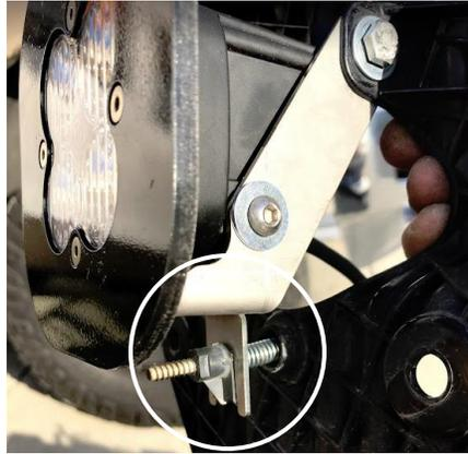
7. Place the OEM fog pocket shroud onto the fog lamp assembly and check the fitment of the light bezel. Adjust the housing bolts and OEM tilt adjuster until desired fitment is attained. Replace the fog pocket shroud fasteners and tighten.
