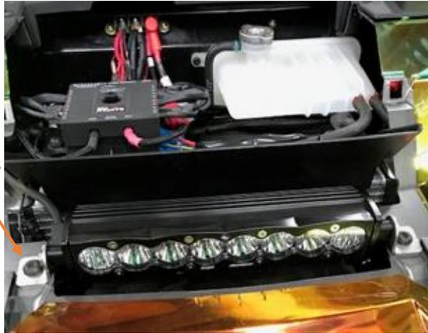
6. Use a 10mm socket and connect the negative and positive terminals of the wiring harness to the positive and negative terminals under the hood or directly to the battery underneath your seat. Do not connect the the harness leads to the far left terminal (this can only take a small amount of amps)
