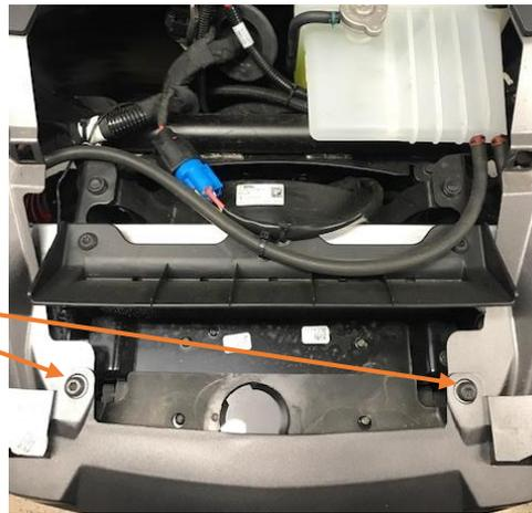
3. Bolt the S8 to the L brackets and tighten
