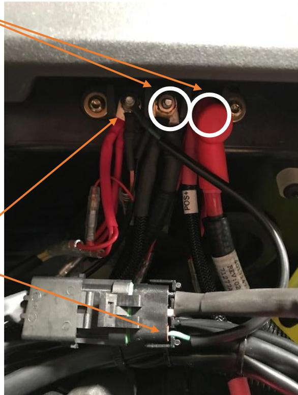
7. Insert the S8 backlight extension into the empty slot on the harness and attach that to the FAR LEFT terminal post to make the back light feature come on with ignition.
