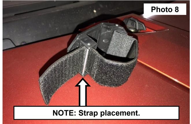
8. Install the 4 straps into the opening in each corner of the windshield. See Photo 9.
