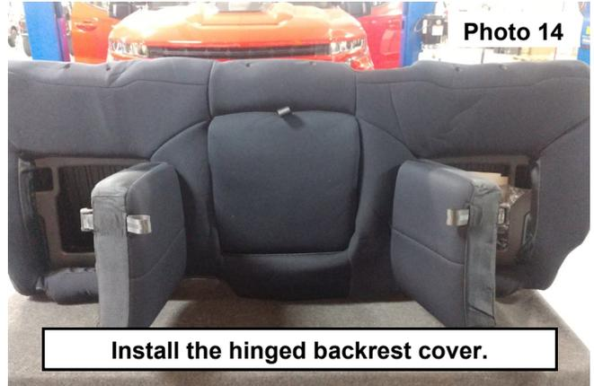
16. Slide the cover onto the backrest tuck the cover around the hinges. Tuck the cover into opening in the back and secure using the Velcro on the inside of the cover. **See Photo 15.**
