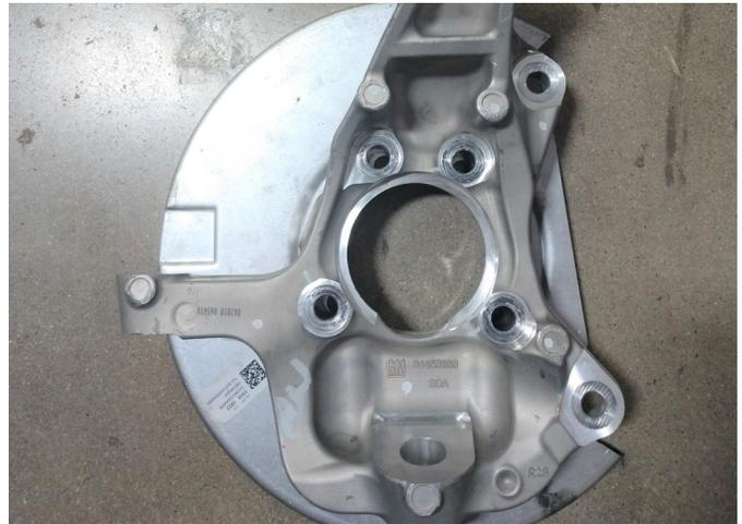
18. Remove the two O-Rings from the OEM spindle and place them on the new Belltech spindle. Attach the hub assembly and dust plate on the Belltech spindle, torque the stock hub bolts to 130 ft lbs. (Ensure the dust plate is aligned as in the OEM position).
