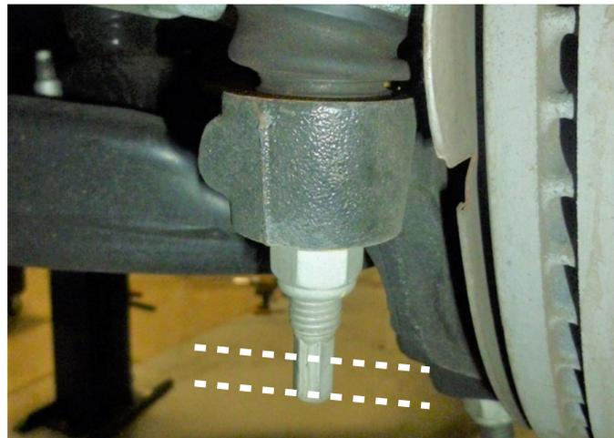
24. Connect the ABS sensor on the side of the Belltech steering knuckle.
