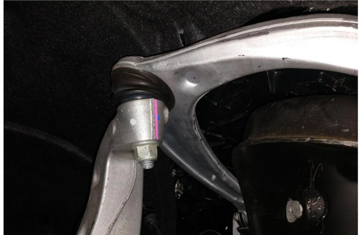
2. Using a 21mm wrench, loosen the tire rod ball joint nut and again keep the nut partially threaded onto the ball joint, free the ball joint from the steering knuckle using the ball joint tool.
