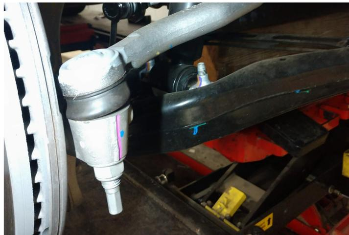
3. Loosen the lower ball joint nut for the ball joint removal using a 24mm socket. It may be helpful to use an hex key inserted in to the lower ball joint to prevent spinning.
