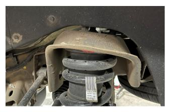
12. Push the lower control arm down until the top of the strut is clear from the chassis then pull the strut out from control arm.
