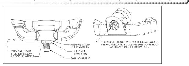
23. Attach the steering tie rod end to the spindle and torque to 37 ft lbs.
