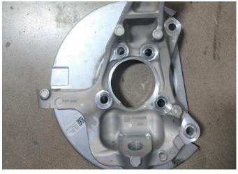
18. Remove the two O-Rings from the OEM spindle and place them on the new Belltech spindle. Attach the hub assembly and dust plate on the Belltech spindle, torque the stock hub bolts to 130 ft lbs. (Ensure the dust plate is aligned as in the OEM position).
