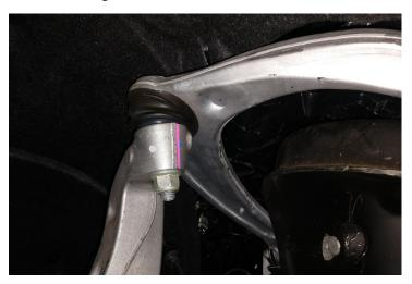
2. Using a 21mm wrench, loosen the tire rod ball joint nut and again keep the nut partially threaded onto the ball joint, free the ball joint from the steering knuckle using the ball joint tool.
