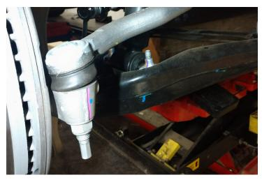
3. Loosen the lower ball joint nut for the ball joint removal using a 24mm socket. It may be helpful to use an hex key inserted in to the lower ball joint to prevent spinning.
