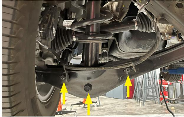
10. Remove the 24mm lower control arm bolt attaching the control arm to the spindle.
