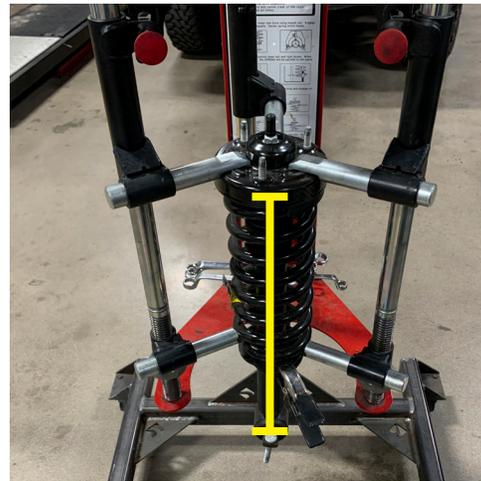
14. Compress the spring until tension is relieved from the strut.
