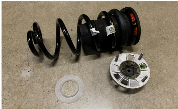
18. Remove the OEM strut from the compressed spring fixture.
