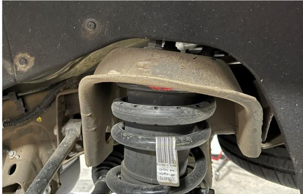
12. Push the lower control arm down until the top of the strut is clear from the chassis then pull the strut out from control arm.
