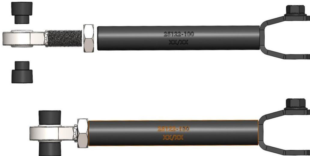
13. Preset the length of the adjustable control arm and set by tightening the jam nut to prevent adjustment from moving during the installation process. To achieve lowering between 3" to 4", set the distance from center to center at 320mm (12.59").
