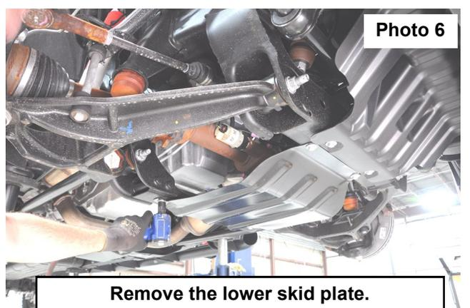
10. Using a 15mm socket, remove the lower skid plate. **See Photo 7.**
