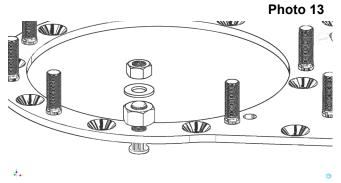
Install the studs in the clocking ring.
