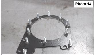
11 studs installed into the clocking ring.
