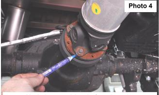
Mark the rear driveshaft at the axle.
