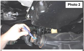
Mark the front driveshaft at the axle.
