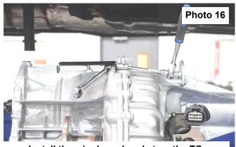
Install the wire loom bracket on the TC.
