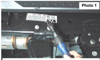
Remove the transfer case skid plate.
