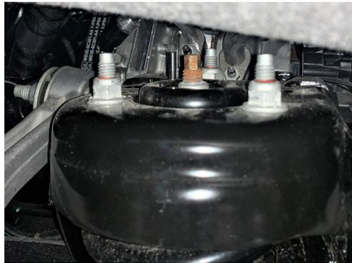
27. Place the lower strut mount onto the lower control arm. Torque the original lower strut bolts and nuts to 66 ft lbs.
