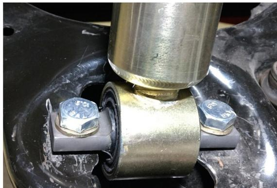
28. Attach the spindle to the upper ball joint. Ensure the CV axle shaft properly aligns into the hub. Torque the upper ball joint nut to 46 ft lbs.
