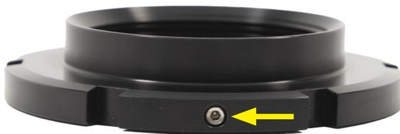
22. Using the provided spanner wrench, turn the bottom spring perch to obtain desired spring perch height, measuring from the top of the perch to the center of the lower bushing. Find the appropriate spring perch height by referencing the tables above. We do not recommend adjusting beyond what is shown on the table as the performance of the shock may decrease greatly.
