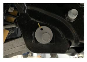
10. Use an 18mm socket to remove the sway bar end link from the lower control arm.
