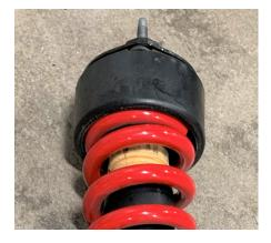
29. Torque the supplied nyloc nut onto the strut, torque to 26 ft lbs. Reference the OE strut markings and ensure the top mount is oriented in the same fashion it was before disassembly.
