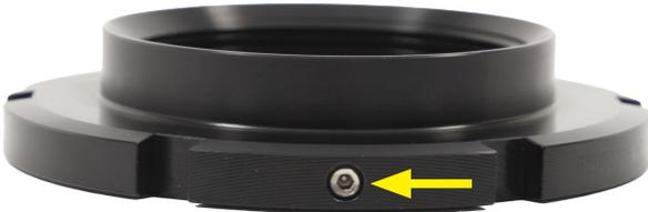
17. Use the provided spanner wrench to turn the bottom spring perch to obtain desired spring perch height. Measure from the top of the perch to the center of the lower mount bushing. Find the appropriate spring perch height by referencing the table below. We do not recommend adjusting outside of the specified height range as the performance of the shock may decrease greatly.
