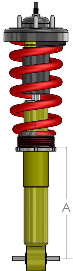
18. Tighten the set screw. Do not over tighten the set screw. Max torque is 1-2 Nm (1.5 ft lbs.)
