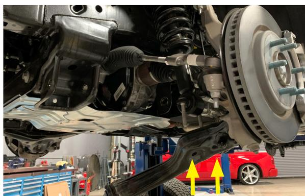
22. Reattach the lower control arm to the frame using the OE alignment hardware. Do not tighten or torque until your vehicle is back on the ground. Torque to 258 ft lbs.
