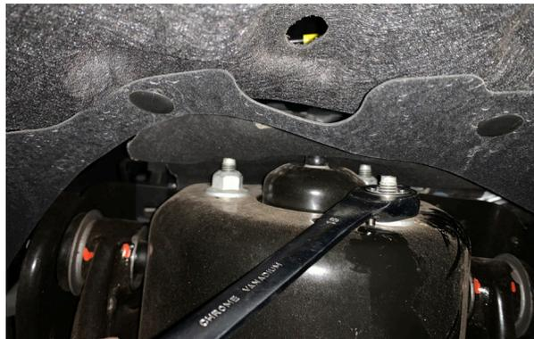
14. Pull the strut assembly out of the chassis strut tower and remove from the vehicle.
