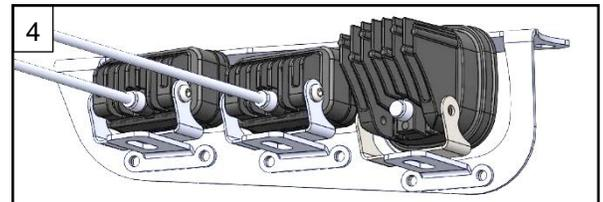
5. Locate the three bolts inside the top surface of either fog light opening in the bumper. Use the T40 bit to remove the bolts, mount the fog light assembly, replace the bolts and tighten. (Driver side shown). Repeat for the other side.
