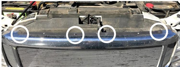
2. With a standard screwdriver (flathead), pry up on the four clips that hold the bottom of the grille on the vehicle. To access the clips, place the standard screwdriver in between the top surface of the bumper and under the grille. The photo below shows the location of the clips. The next photo shows the clip.
